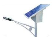
Solar Street Light are independent light source which are wireless and not connected to any grid. It works on energy stored in his batteries, generated through Solar Panels. Most efficient solutions for lighting problems in remote areas
